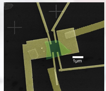
Figure 2. \text{MoS}_2 device in a Hall bar configuration. Green is the 5 nm thick \text{MoS}_2 flake; gold shows the normal metal contacts.
