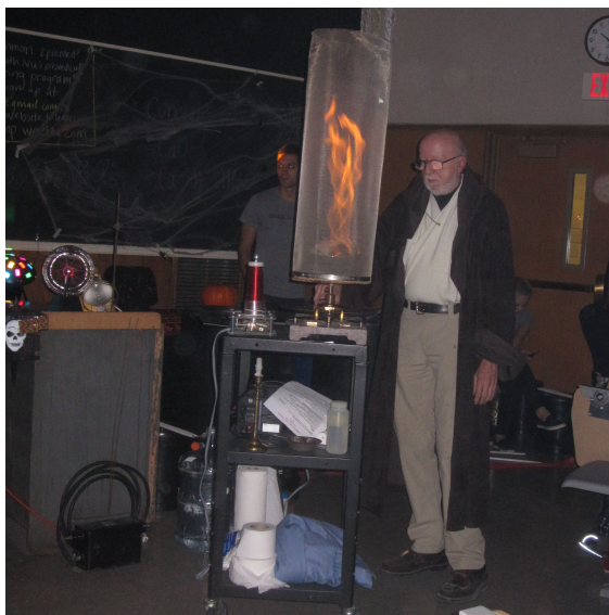
Pillar of Fire- rotating tube of mesh creates a tornado of fire from small alcohol flame.
